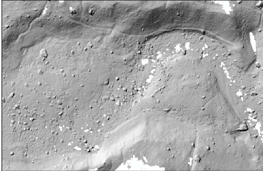
FIGURE 3-5 HILLSHADE EXAMPLE. ONCE A RASTER IS CREATED WITH ELEVATION DATA, A HILLSHADE CAN BE CREATED. THIS TOOL CREATES A SOURCE OF ILLUMINATION TO BETTER VISUALIZE OBJECTS AND TERRAIN.
