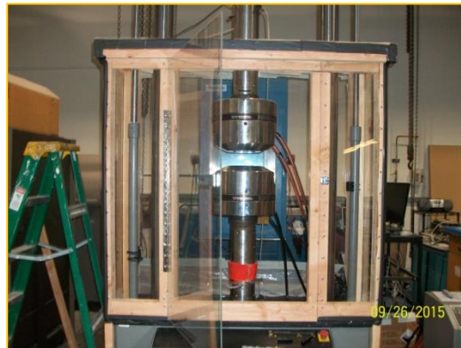
Figure II: Testing Isolation- Chamber
