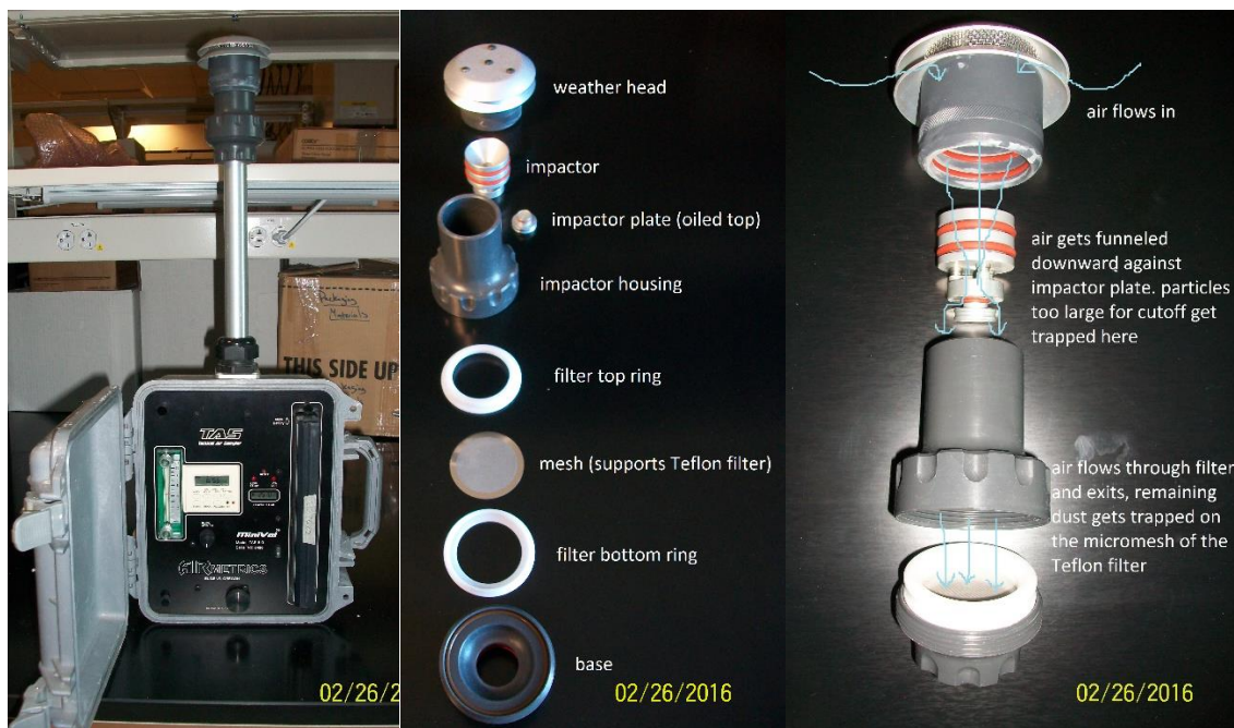
Figure V: MiniVol Filter Assembly (PM 2.5)
