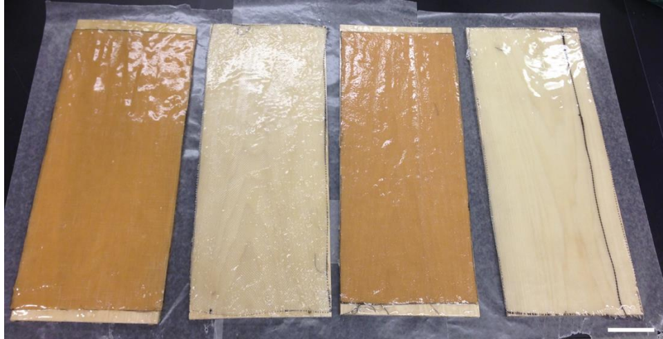
Figure 15: From left to right, G-Fl, G-Fi, E-Fl, and E-Fi FRP composite strengthened wood (5cm scale bar).
