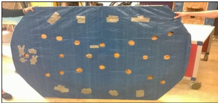
Figure 14: Skirt holes patched with duct tape
