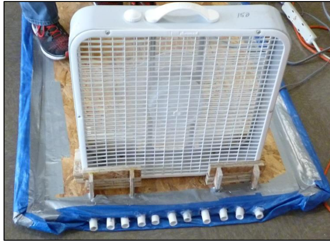
Figure 15: Piping added to the back of a craft to improve propulsion
