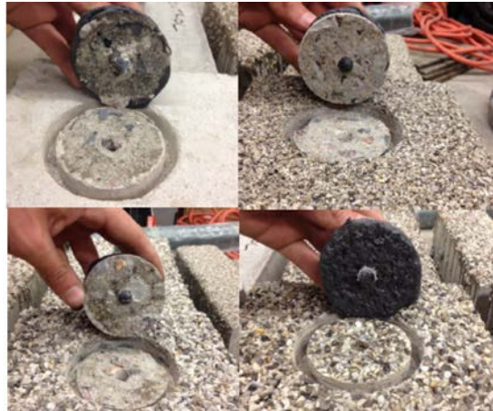
Figure-38 Bond test for quality control
