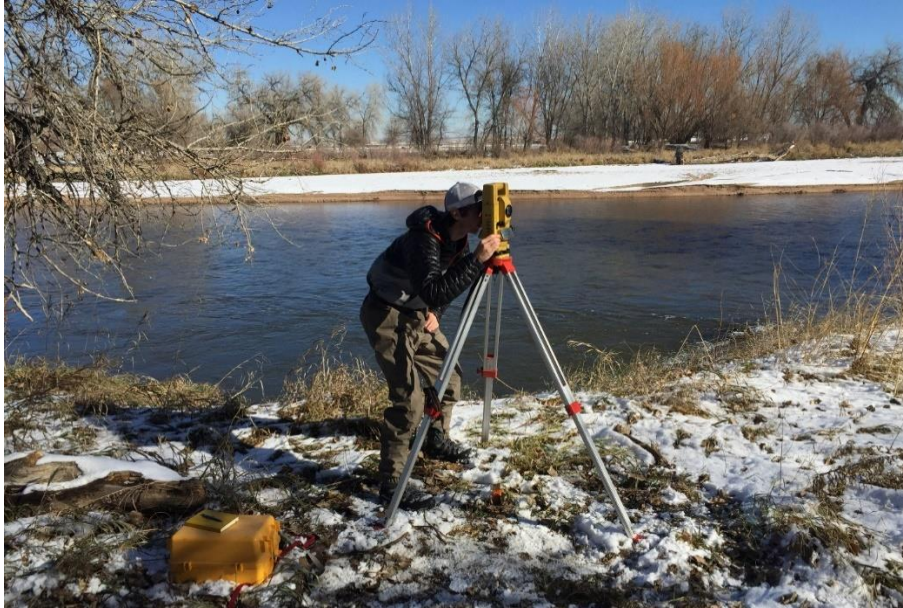
Figure 5. The setup of the total station to get distance and angle measurements of varying locations. In the background of the photo is the large sand bar as well as a dense population of willow bushes.
