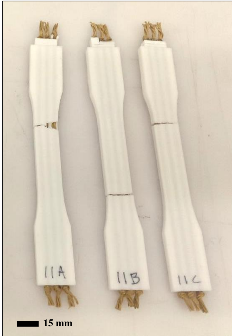
Figure 13. Flax-reinforced tensile composite specimens, post-break.
