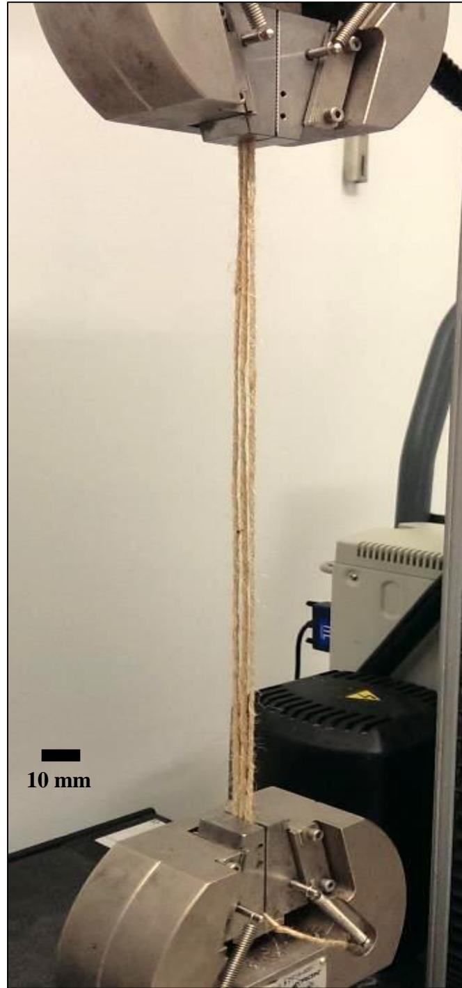
Figure 7. Sample of three (3) jute fibers during mechanical tensile strength testing.
