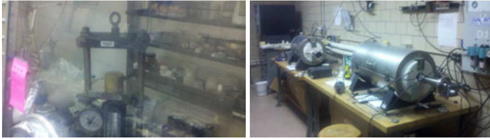
Figure 3.2: Left: hydraulic press used for making TMAs powder pellets. Right: horizontal furnaces used for solid state synthesis of TMAs. The foreground furnace has the rotating sample attachment inserted.
