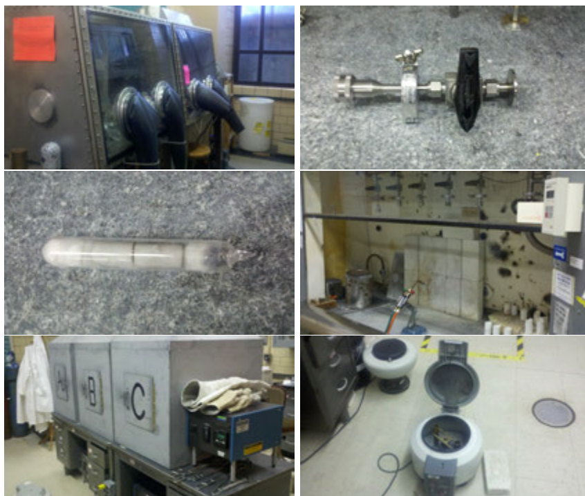
Figure 3.4: Top left: dry nitrogen glove box used for air work with air sensitive elements. Top right: detachable valve unit for the glass bench which can be taken into the dry glove box. Middle left: doubly-sealed \text{SiO}_2 ampoule representative of those used for synthesis of crystals containing highly volatile, toxic or air sensitive constituents. Middle Right: double-tube and valve assembly together. Bottom left: "box" furnaces used for high temperature sample synthesis. The furnaces are inside a vented metal enclosure to guard against the possibility of explosive accidents. Bottom right: centrifuge used for decanting excess liquid from the growth.
