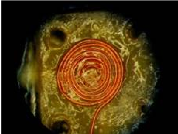
Figure 2.2: Example of a flat “pancake” coil in which a wire is wrapped in-plane around a central point increasing the radius for successive turns.
