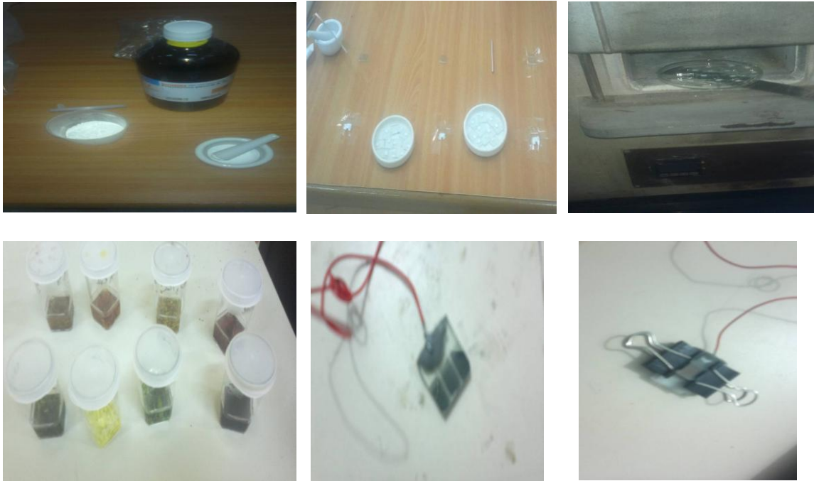
Fig.3.1. Steps of the DSSC assembly.
