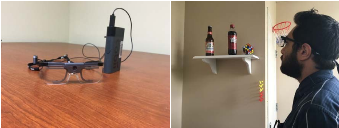
Figure 1. Eye-tracking glasses with portable battery pack (left) and the eye-tracking glasses as they would be worn during an in vivo assessment of attention (right).
