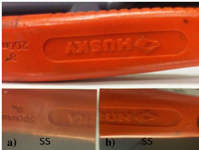
Figure 2.4: a) Unpolished and b) polished SS Sheet. The top photo is the object reflected in a) and b)
