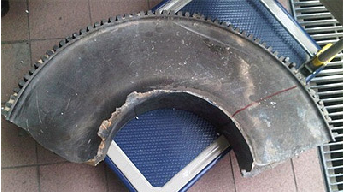
Figure 1.2 - Large Piece of a Fracture Disk from a Qantas Airbus A380 [3]
