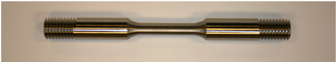
Figure 3.7 - Specimen Used for High Temperature Tensile Tests
