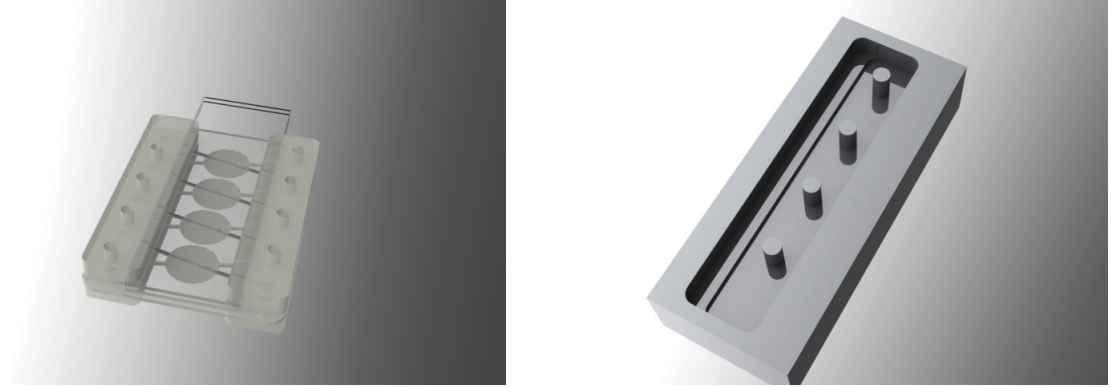
Figure 25: Assembly of membrane with slides and tubing connectors (left) with tube holder mold (right)
