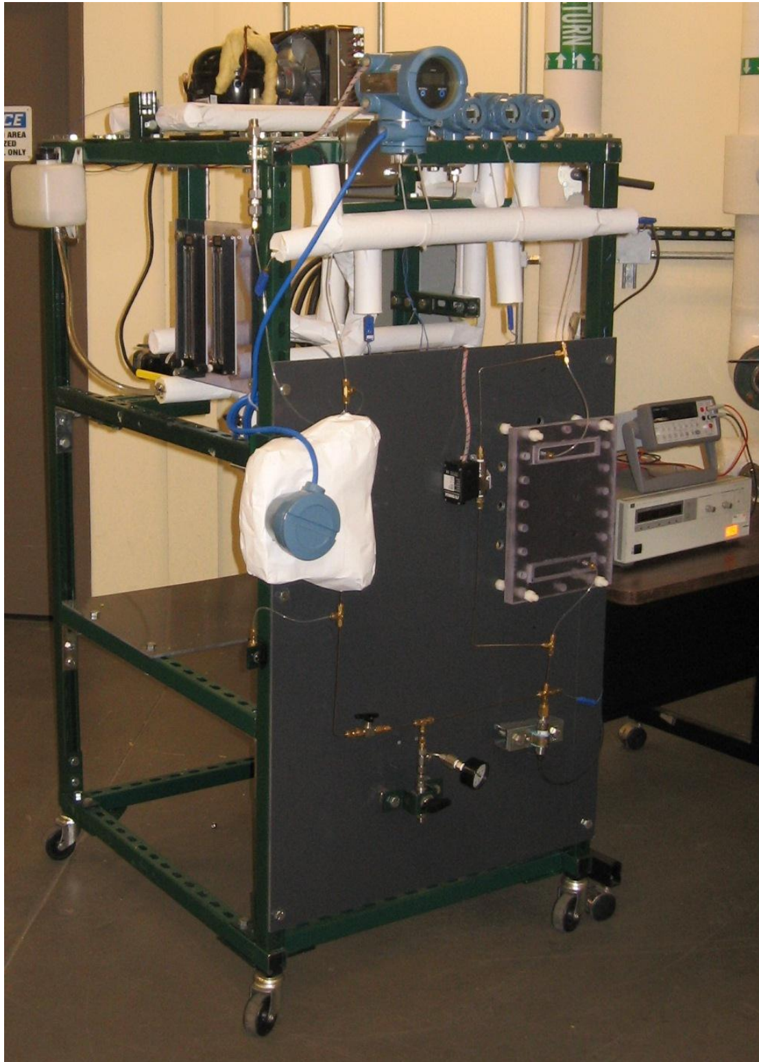
Figure 4.4: Microscale Phase Change Internal Cooling Test Facility (environmental enclosure and expansion tank not shown for clarity)
