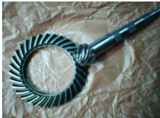
Figure 1-6: Typical high-power-density gear, made of carburized Ferrium® C61 [44].
