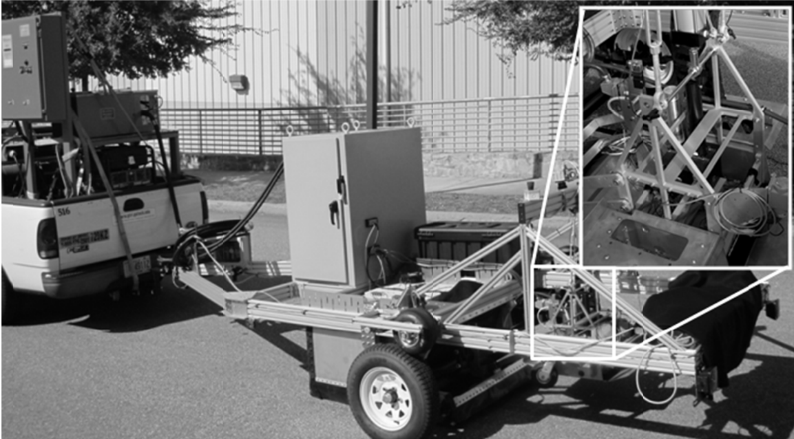
Figure 16: Picture of Prototype Crack Sealing Hardware with Detail of Applicators
