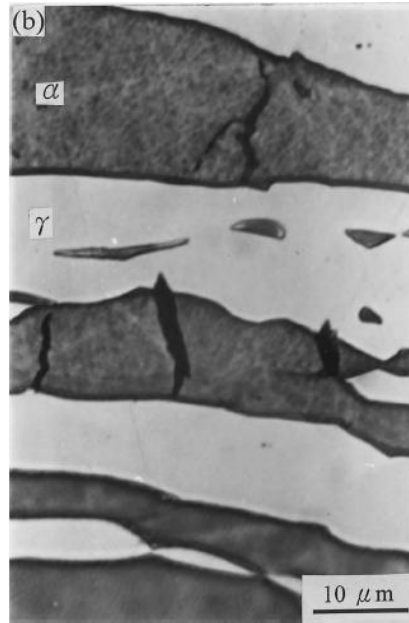
FIGURE 2.17 Micrograph of DSS 2205 after testing in 26 wt.% NaCl solution of pH = 2 and at -400 mV (SCE). [34]
