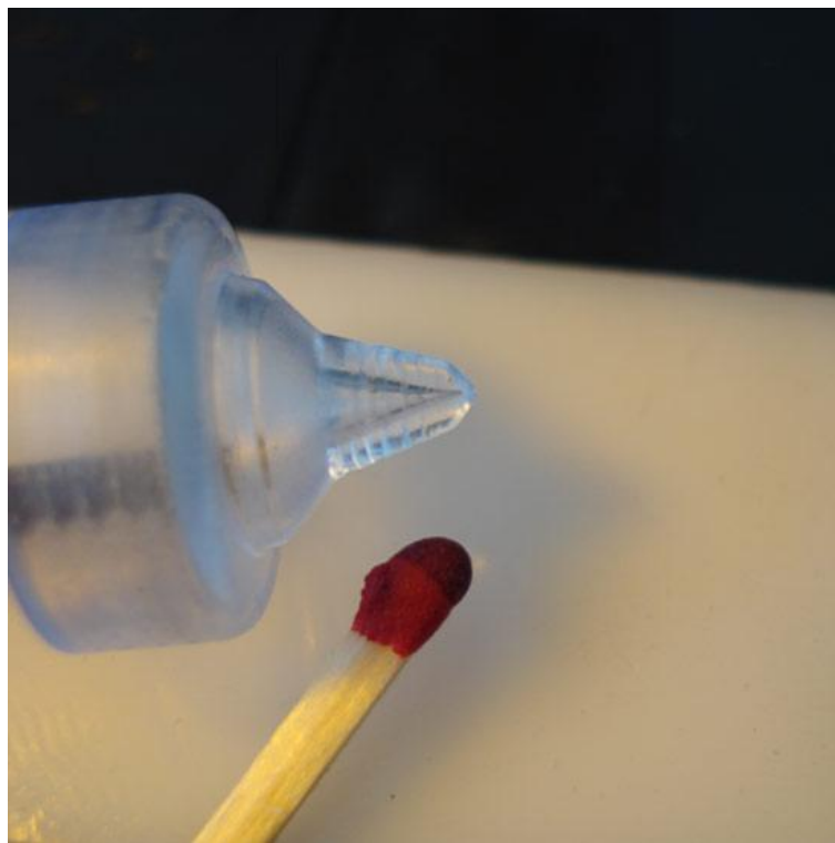
Figure 1.2: Micro milled orifice (0.07 mm diameter) in a nozzle for use in biomedical applications (Microlution, Inc.).
