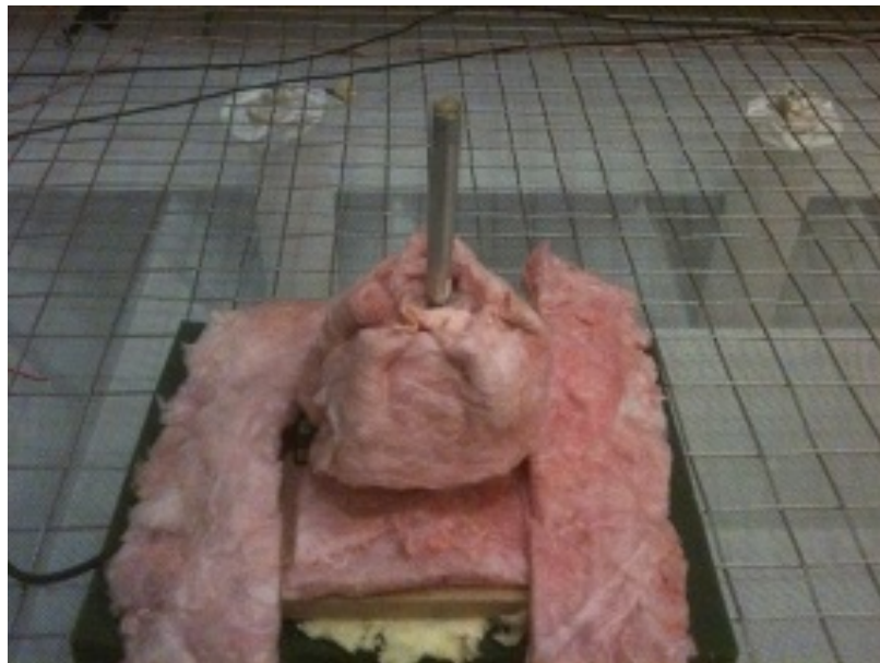
Figure 55: Directivity test setup with shielding
