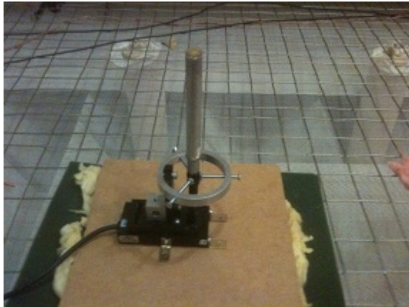
Figure 54: Directivity test setup without shielding
