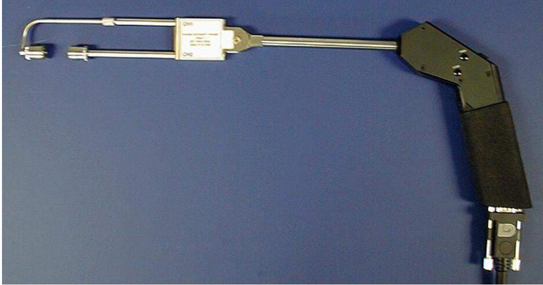
Figure 4: Directional microphone using two inphase microphones [10]
