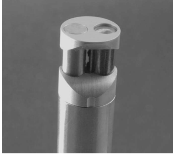
Figure 8: Microflow directional microphone fully packaged [29]
