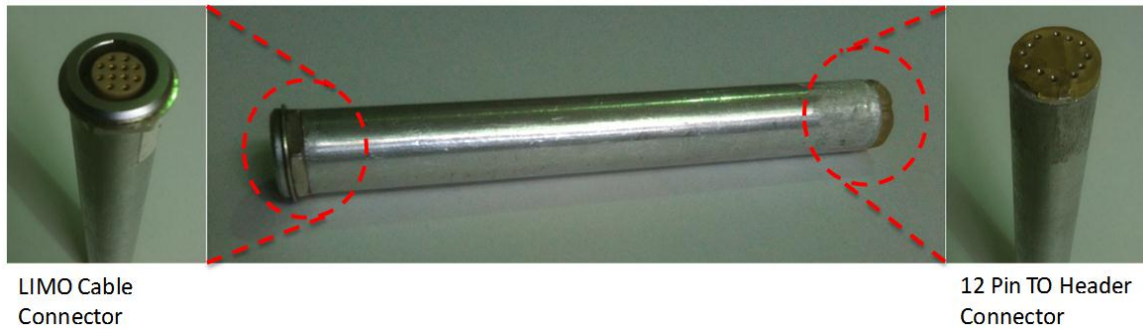
Figure 82: IO Map preamplifier tube with connection ports shown
