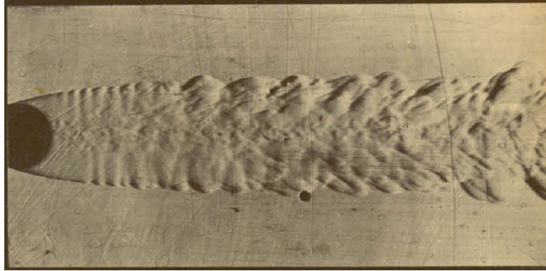
Figure 1.3: Schlieren photograph of a high dilatation ratio ( \rho_u/\rho_b ) bluff body-stabilized flame, showing wake symmetry (reproduced from [28]).
