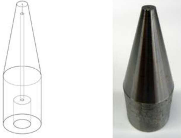
Figure 27: a) Schematic of the high pressure constricting nozzle b) High pressure constricting nozzle used on system
