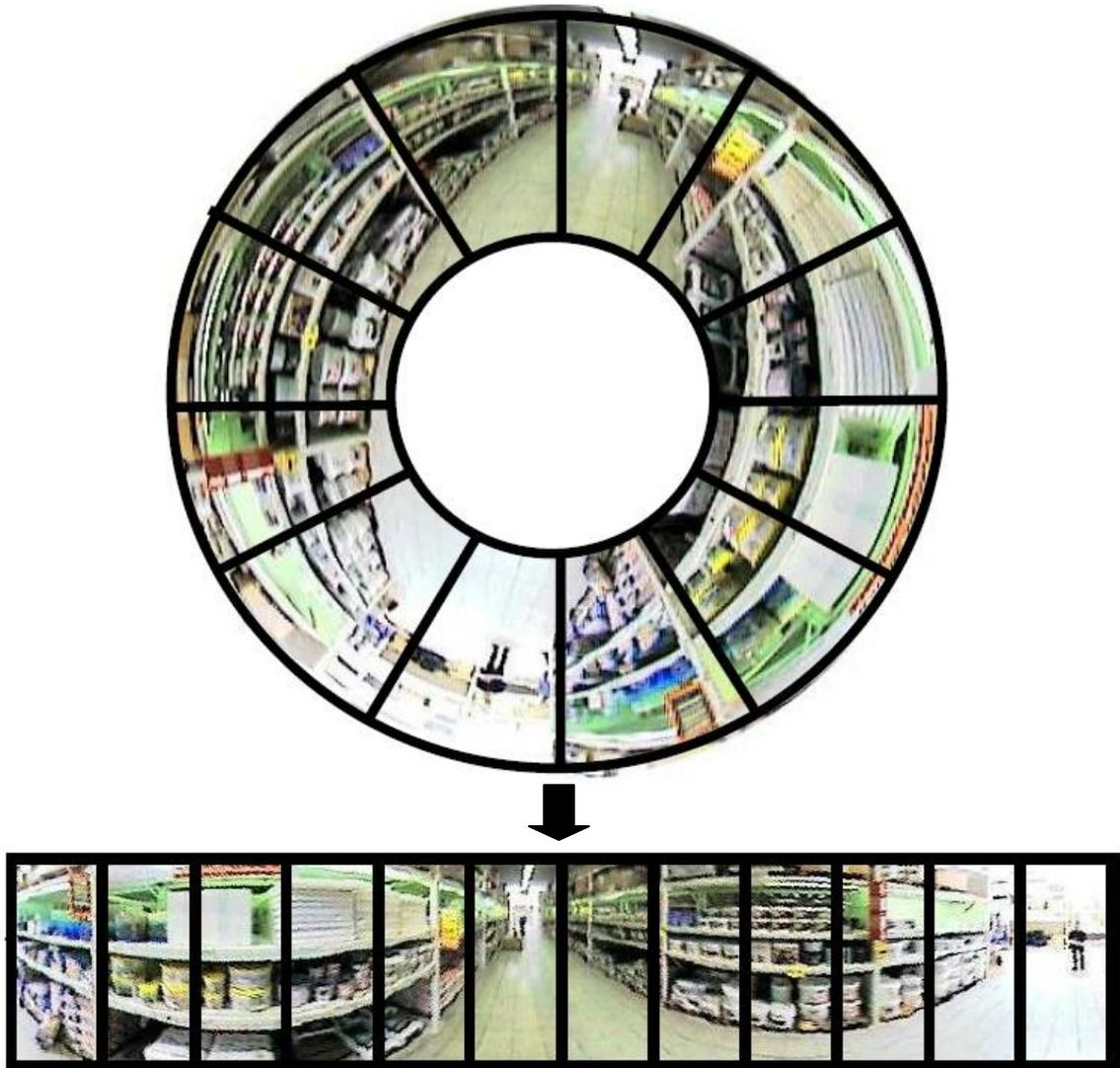
**Figure 2:** Captured Catadioptric stereo image and the unwrapped panoramic image [28]
