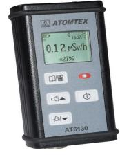
Fig. (3.1): AT6130 Radiation Monitor
