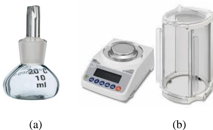
Fig. (3.4): (a) The 10ml pycnometer (b) The HX-Z analytical balance
