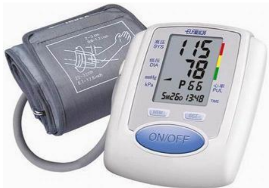
Fig. 3.3: Arterial Blood Pressure and Heart Pulse Rate Meter, model WS- 300 (Instructions manual for Automatic Digital Electronic Wrist Blood Pressure, 1998a)
