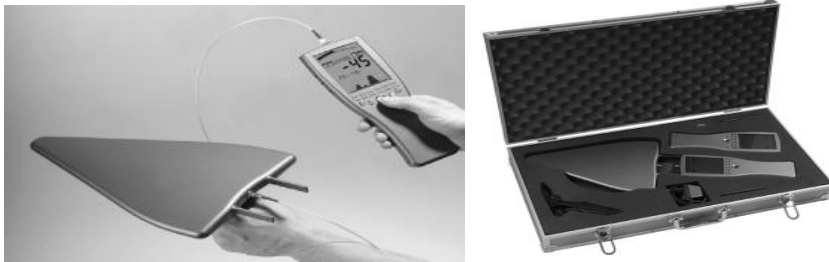
Fig. 3.1: Spectran RF 6080 (Instructions manual for spectran RF 6080, Aaronia AG, Germany, 2007).
