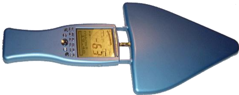
Fig. 3.1: Spectran of radio frequency (RF) 6080
