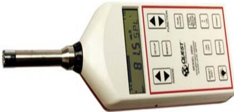
Fig. 3.6: Sound level meter model 2900
