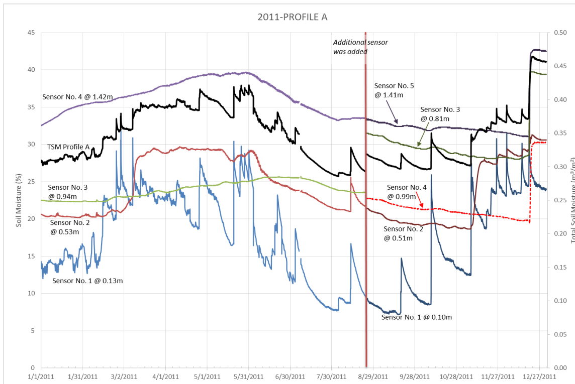
Figure D 2. Soil moisture and total soil moisture for profile A in 2011.
