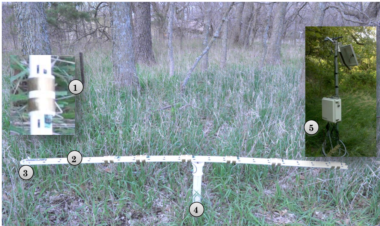
Figure 3. 2. Sentek EnviroSCAN soil moisture profiler system customized for our application. The 6 pairs of gold-colored rings (No. 1) constitute the capacitance sensors set at 6 different depths that slide along a plastic type cartridge (No.2) and all connected to an electronic interface (No. 3) that communicates with a centralized external data logger (No.5). The cartridge is then placed inside the access tube (No. 4, white PVC pipe).
