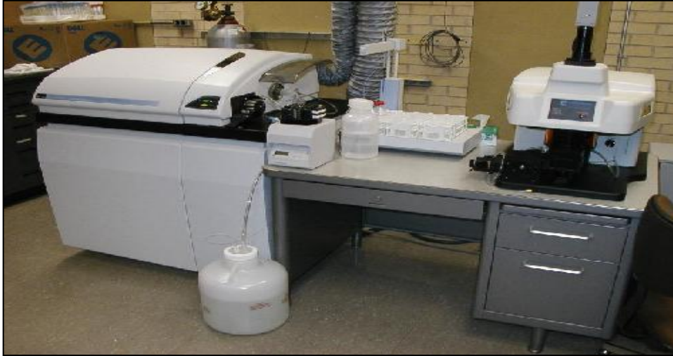
Figure (3.5): ICP – MS (Perkin Elmer Elan 9000) device
