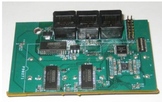
Figure 7.1. (a) University of Colorado PV array and (b) PCB for sub-module data collection
