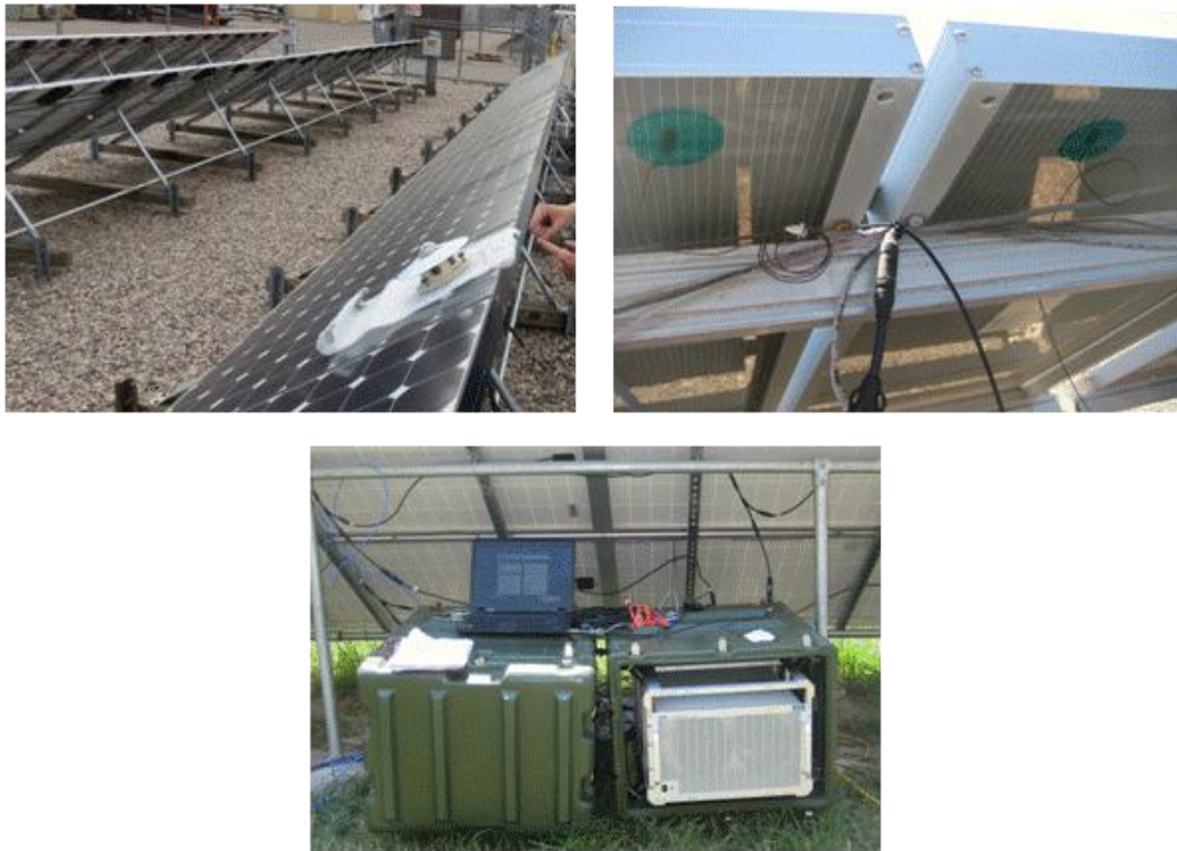
Figure 3.4. Pyranometer (top left), temperature sensors (top right) and multitracer system (bottom)
