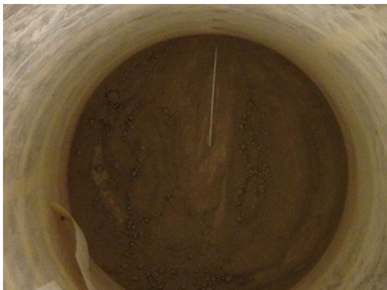
Figure 6.14: View of needle location as soil was being removed after the experiment was finished
