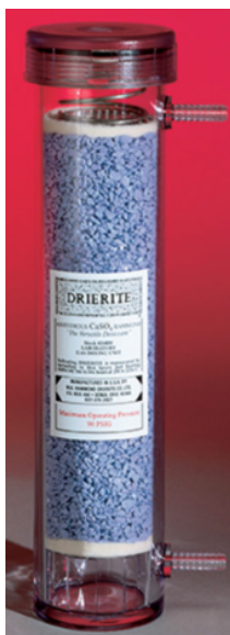
Figure 6.11: Drierite-filled laboratory gas drying unit
