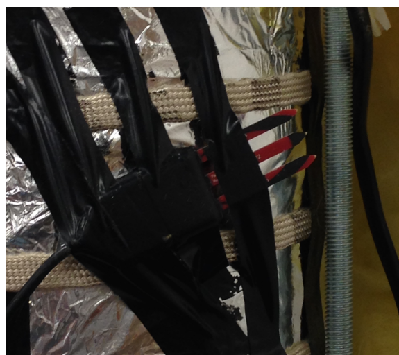
Figure 6.7: Temperature sensor attached to the outside of the cylinder in order to record the heating tape temperature
