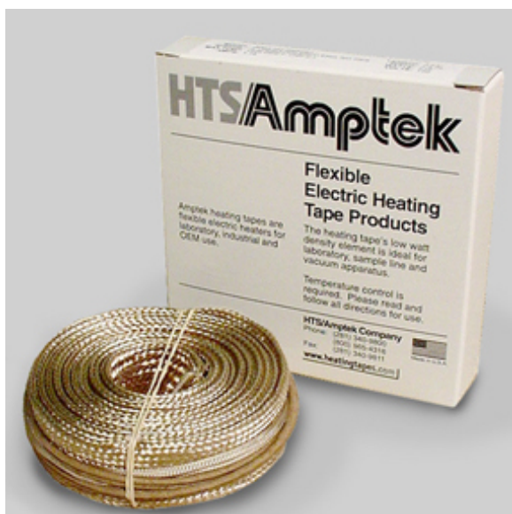
Figure 6.5: HTS/Amptek heating tape. The heating element is multi-strand resistance wire, braided with AMOX yarn and knitted into the serpentine shape.
