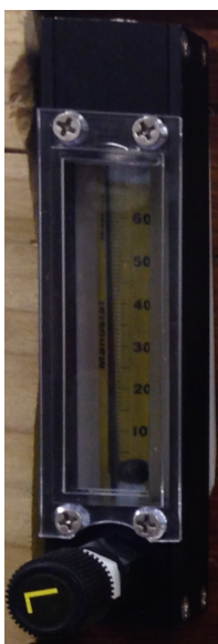
Figure 6.9: Riteflow flow meter: 65mm long with glass float
