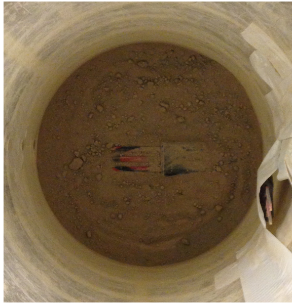
Figure 6.21: View of dielectric sensor location as soil was being removed after the experiment was finished
