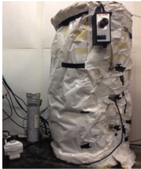
Figure 6.4: The cylinder was insulated with fiberglass
