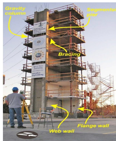
Figure 7-2. View of the building tested at UCSD (Moaveni et al., 2011).
