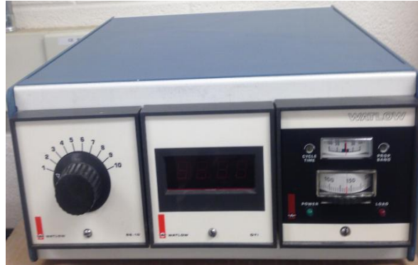
Figure 4.9: Temperature controller (WATLOW 88-10).
