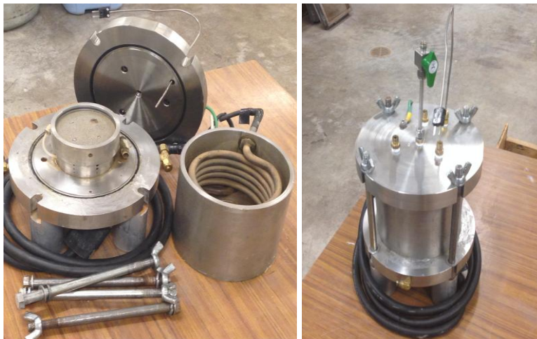
Figure 4.8: Pictures of the pressurized reservoir containing the heating coil.
