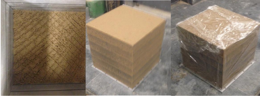
Figure 3.6: Cubical specimen of Bonny silt after compaction: (a) Compacted lift scarified; (b) Soil specimen; (c) Soil specimen wrapped in plastic.
