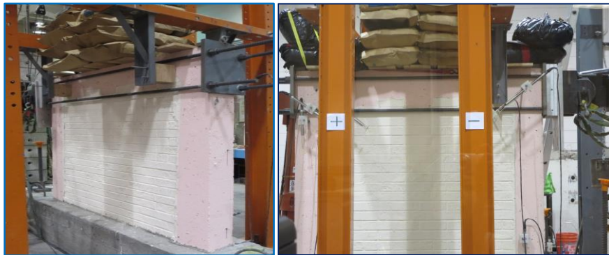
Figure 3-47. Nguyen CM Wall 2 experimental test setup
