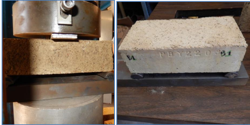
Figure 3-18. Unit flexural test
