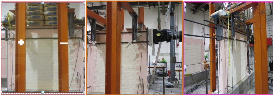
Figure 3-41. Test setup with sand bag as vertical roof load
