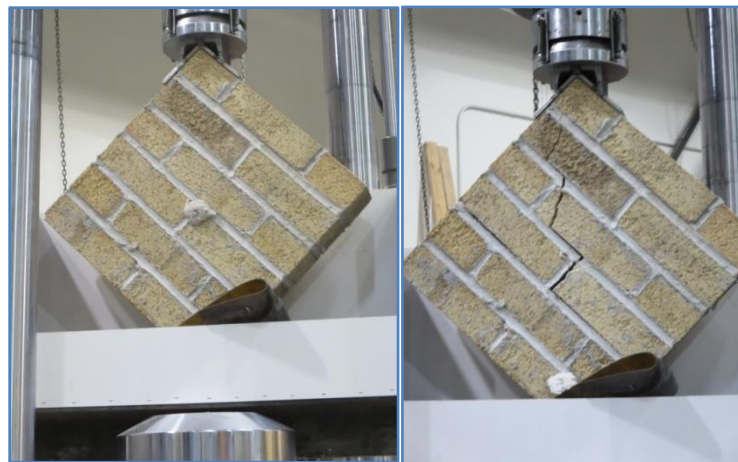
Figure 3-26. Diagonal Compressive Shear test
