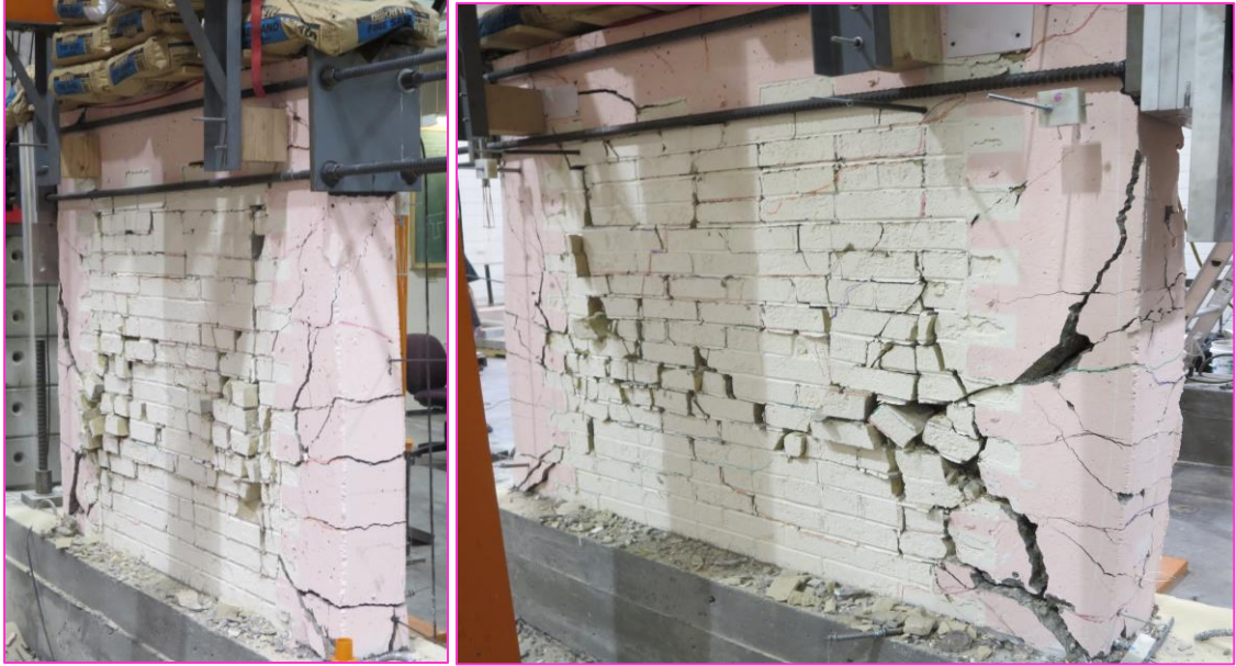
Figure 3-59. CM shear wall 1 failure mechanism
