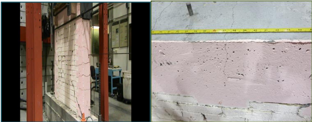
Figure 3-44. Nguyen CM Wall 1 experimental test result on column and beam
