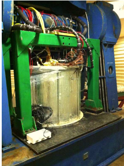
Figure 5.2: a single energy foundation SSI experiment mounted on a 400 g-ton centrifuge bucket.
