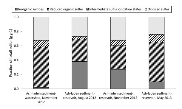
Figure 4.6: Fractional sulfur oxidation states in ash-laden sediment collected from stream banks and the reservoir bottom are grouped into absorption regions.
