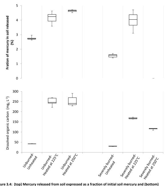
Figure 3.4: (top) Mercury released from soil expressed as a fraction of initial soil mercury and (bottom) organic matter released from soil measured as dissolved organic carbon as a function of heating.
