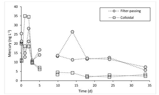
Figure 5.4: Filter-passing and colloidal mercury in microcosm pore water as a function of time in duplicate microcosms. We lost the 7 d samples.
