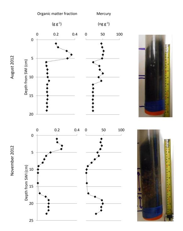
Figure 4.3: Organic matter and mercury profiles in reservoir cores collected in August and November 2012. Organic matter content was the best indicator of the deposited ash-laden sediments in the reservoir. In the November core, a gravel layer separated the ash-laden sediment and the native reservoir sediment.
