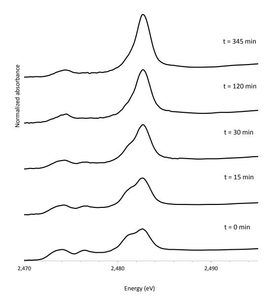
Figure 3.6: Sulfur XANES spectra in unburned soils (Area B) subjected to increasing duration of heating at 225°C reveals an increase in the oxidized sulfur peak above 2,480 eV and loss of reduced and intermediate oxidation states below 2,478 eV.
