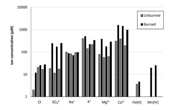
Figure 3.5: Measured ion release increased following heating of unburned soil collected from Area-B at 225°C. The greatest increase occurred for manganese (67-fold), the low initial value does not show up on a log scale.
