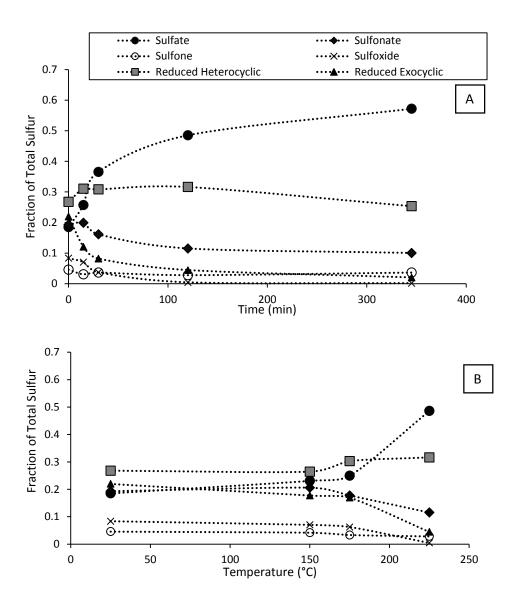
Figure 3.7: Sulfur speciation in unburned soil (Area B) as a function of (A) exposure to increasing temperature for 2 h intervals and (B) increasing duration of exposure to 225°C. The soil heated at 2 h for 225°C is shown in each series.
