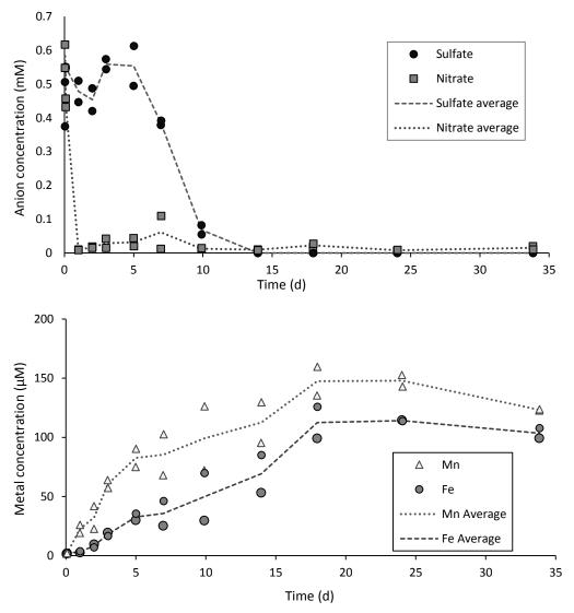
Figure 5.2: Concentrations of redox-sensitive anions and metals as a function of time in microcosms.
