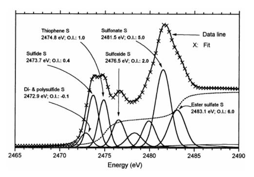
Figure 1.5: Sulfur X-ray absorption near edge structure (XANES) spectra is de-convoluted using linear fitting of Gaussian curves centered at the absorption energy of a particular oxidation state. Reduced species occupy the low-energy range (< 2476 eV) and oxidized species occupy the high-energy range (> 2479 eV). Figure from Vairavamurthy (1998).
