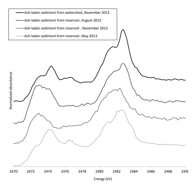
Figure 4.5: Sulfur XANES spectra collected from river bank and reservoir sediments at three time points after deposition.
