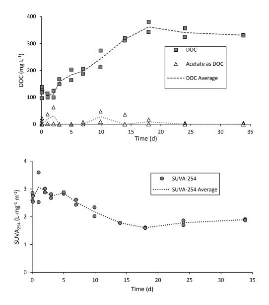
Figure 5.3: Dissolved organic carbon (DOC) and specific ultraviolet absorption (SUVA<sub>254</sub>) of pore water as a function of time are shown in duplicate microcosms DOC and SUVA<sub>254</sub> are shown after correction for acetate. Acetate is shown as its DOC contribution.
