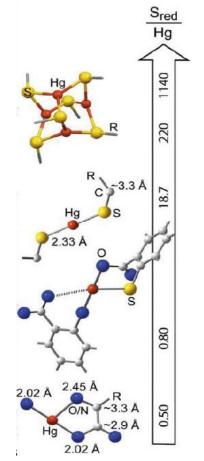
Figure 1.3: Mercury binding coordination dependents on the ratio of reduced sulfur to mercury (S<sub>red</sub>/Hg). Figure from Nagy *et al.* (2011).
