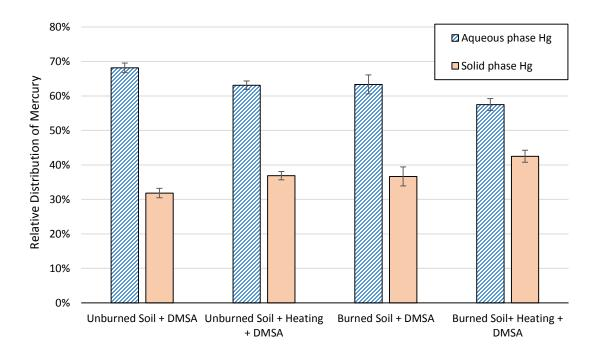
Figure 3.8: Mercury distribution following competitive ligand exchange with *meso*-2,3-dimercaptosuccinic acid (DMSA). Heated and unheated soils are confirmed to be statistically different (*t*-test, p < 0.05). The recovery of mercury in the vials accounted for native and added mercury mass and was 87 ± 10 % (n = 12).
