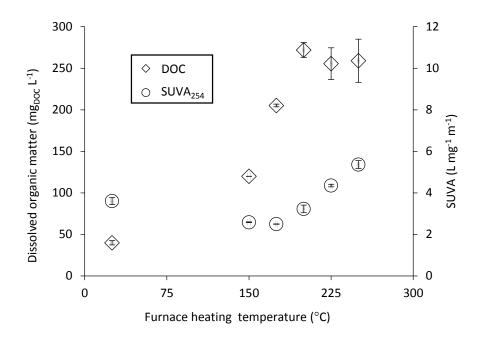
Figure 3.3: Dissolved organic matter measured as carbon (DOC; left axis) and specific ultraviolet absorption (SUVA<sub>254</sub>; right axis) as a function of furnace heating of unburned soil from Area B. Error bars represent the standard deviation of triplicate experiments.
