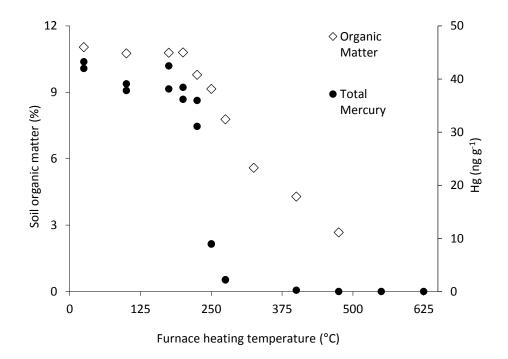
Figure 3.2: Temperature dependence of soil organic matter (left axis) and mercury (right axis) loss from unburned soil from area A over a range of temperatures for 2 h.
