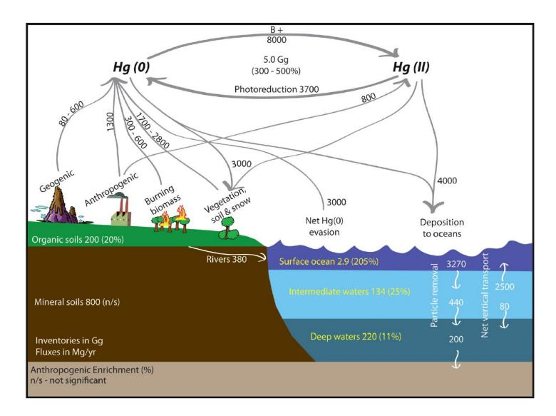
Figure 1.1: Current estimates for global mercury storage and fluxes. Figure from Driscoll et al. (2013).
