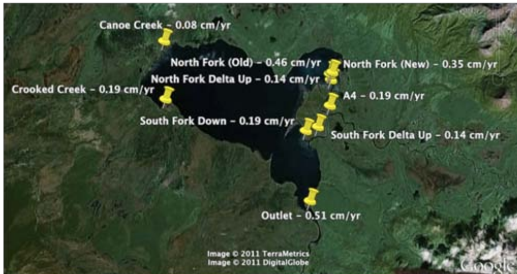
Figure 4.1: Map of Black Lake Depicting Sample Locations and Sedimentation Rates (Google Earth Pro, 2011)
