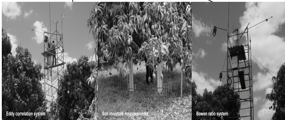
Figure 4.4 Measurements of radiation and energy balance; soil moisture; and reference evapotranspiration in mango orchard.
