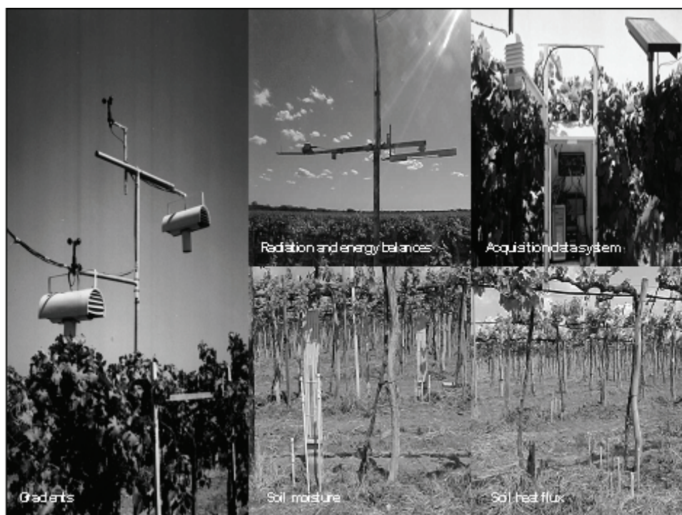
Figure 4.2 Measurements of gradients of air temperature, vapour pressure and wind speed; incident and reflected shortwave; net radiation; acquisition data system; and soil moisture in Bowen ratio system of wine grape.
