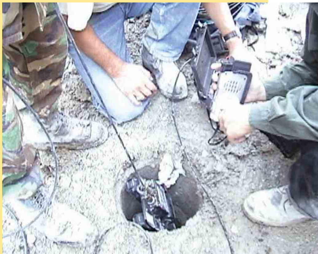
A view of the Inuktun micro-VGTV robot being inserted into a sewer pipe at the World Trade Center site in an attempt to locate an entry to the basement. Note the small size of the robot, the use of a tether as a safety line for the vertical entry, and the use of a camcorder to display the video because of better resolution than the manufacturer's display. This is the only external view of the robots that was allowed to be photographed at the WTC site.
