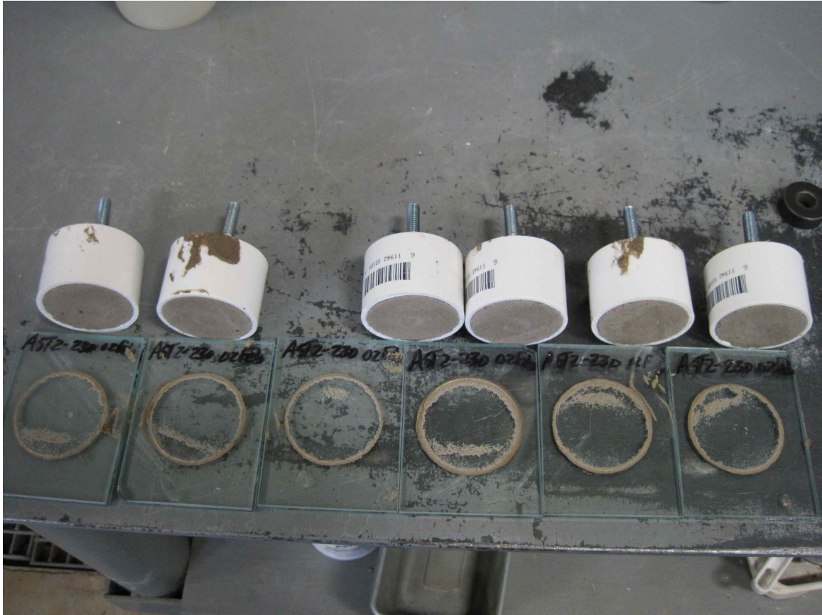
Figure 6.1.16: CSA cement mortar 1 plus polymer 2 with p/c = 0.3 displaying failure mode AF/S, failure at bond line, following pull-off testing over glass substrate after curing for 7 days at ambient laboratory conditions
