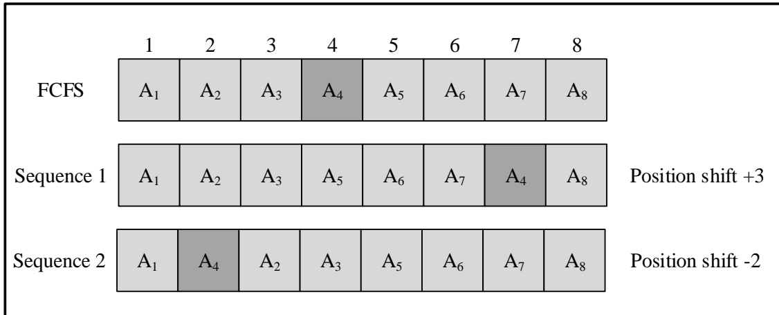
Figure 19: Representation of Position Shift Concept
