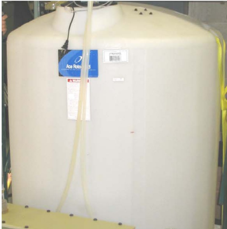
Figure 3.15: Desiccant Storage Tank
