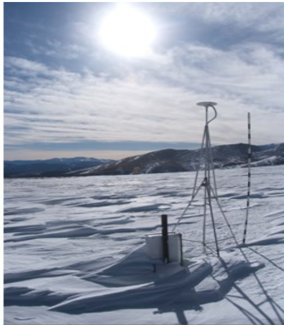
Figure 2.5: Modern GPS-Enabled Snow Gauge at Niwot Ridge, CO (NCAR 2011)
