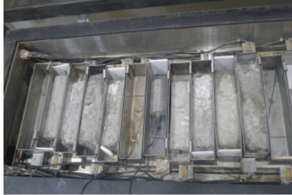
Figure 3-10 Logan Rapid Freeze-Thaw Chest
