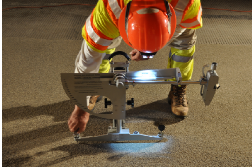
Figure 4-14 Completion of Skid Test (3:00 AM)
