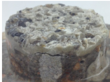
Figure 5-6 MMA Failure plane
