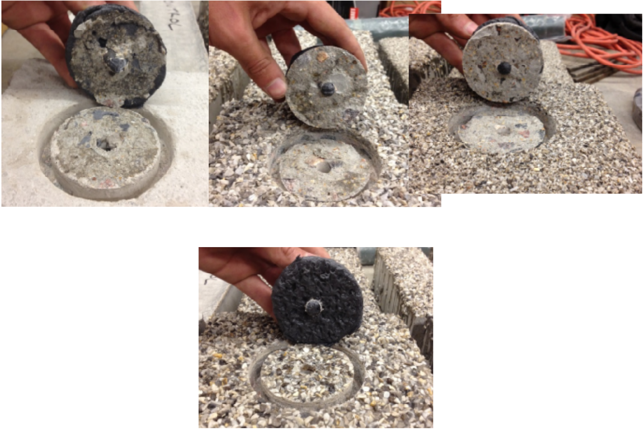
Figure 5-3 24 hr. Bond Test Results (from top to bottom, left to right) Control, Polyester, Epoxy, MMA
