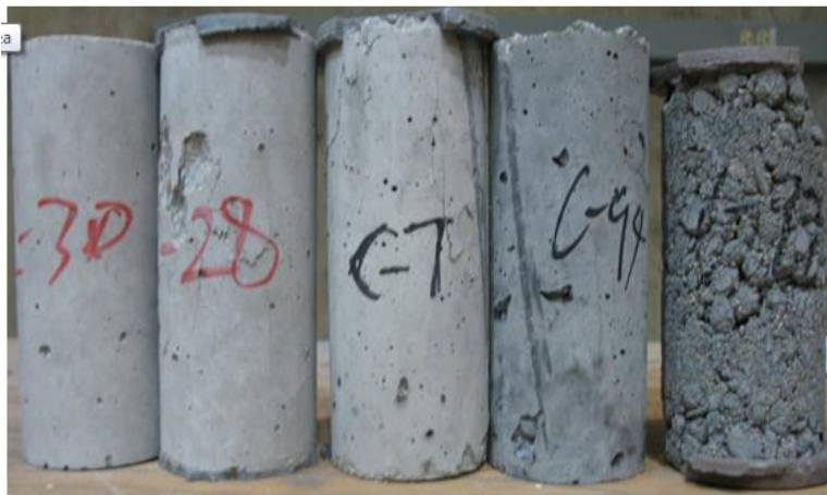
Fig. 63. Surface smoothness variation with increasing CNT dispersion period (CNT content = 0.75% of weight of cement)
