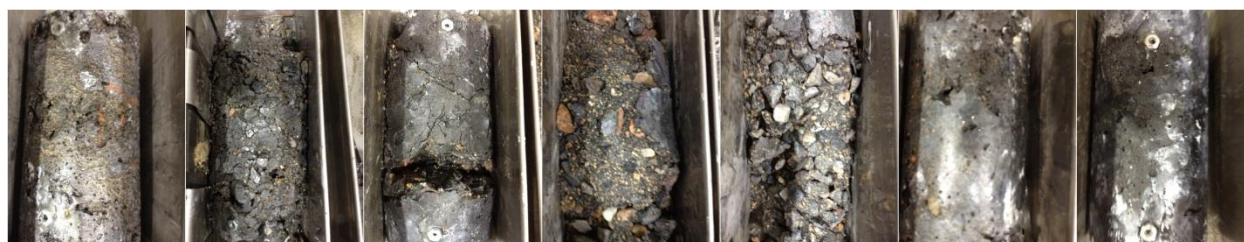
Fig .71 CNT concrete after 300 cycles of freezing and thawing
