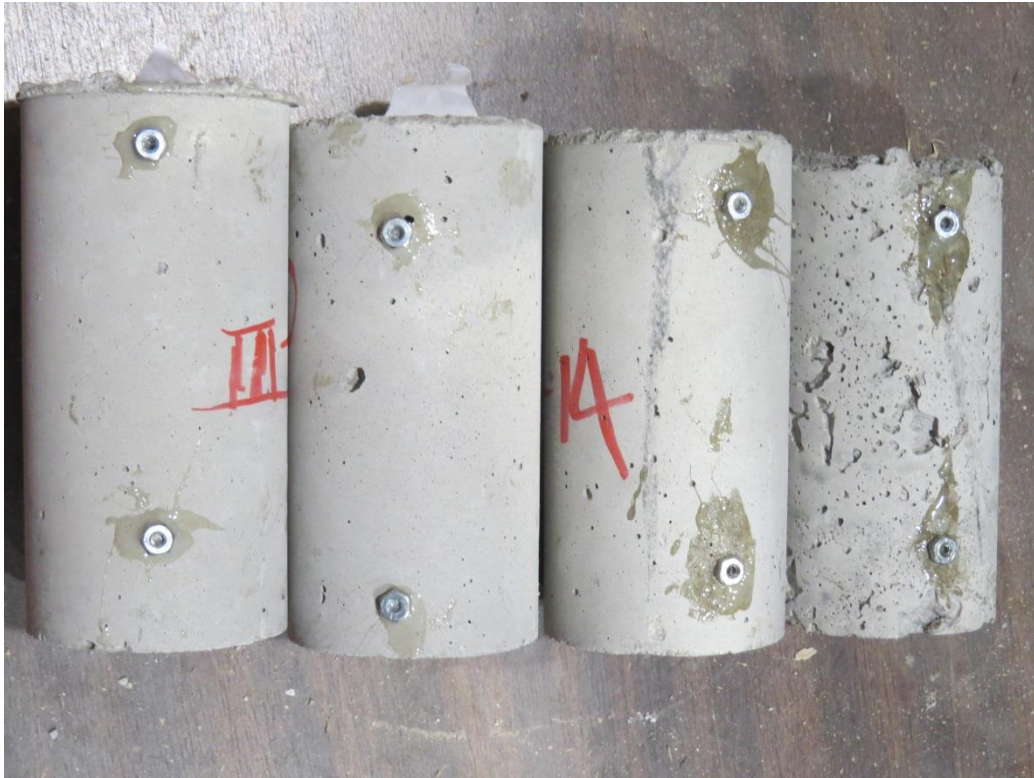
Fig. 10. Bolts Attaching to Specimen for convenient use of Dial Gauge
