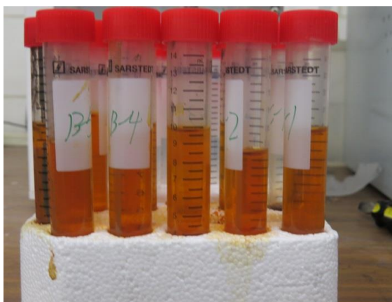
Fig. 66. Mixing Concrete Powder with Cl 2 Solution
