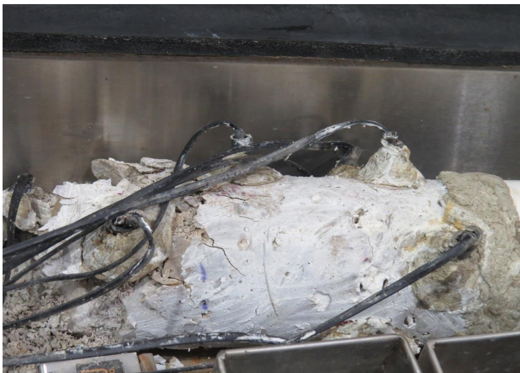
Fig. 9. Sensor buried in different depth of sample specimen
