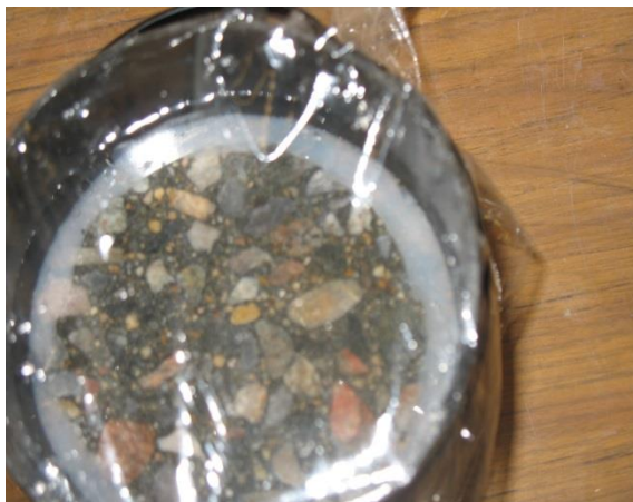
Fig. 64. Concrete Specimen with NaCl Solution on top
