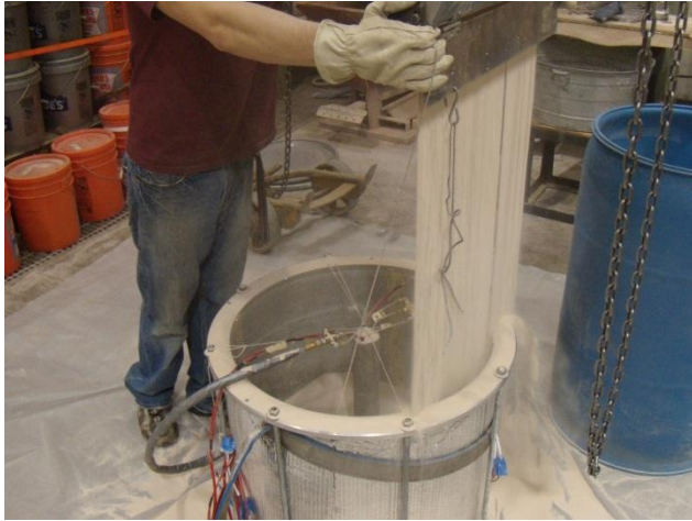
Figure 5.1.1-1 Air pluviation using a sand hopper.
