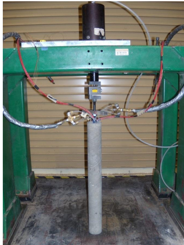
Figure 4.3.1-2 End-bearing foundation prior to thermal and mechanical testing.
