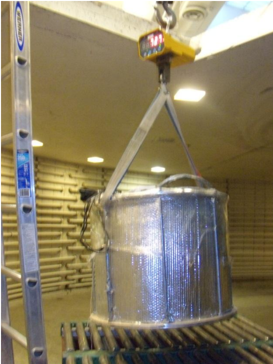
Figure 5.2.1-1 Lowering of the soil container onto the roller cart in the centrifuge chamber with hanging scale.
