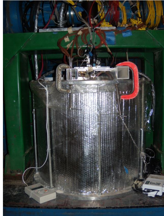
Figure 5.2.1-2 Soil container in place with all instrumentation prepared for testing.
