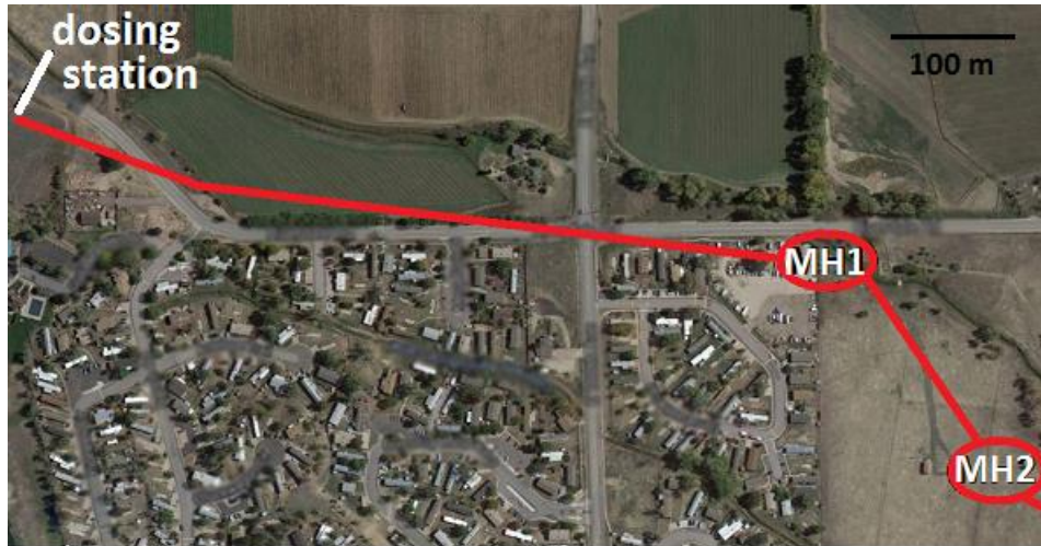
Figure 5.1: Map of manholes and peroxide dosing station. Red line indicates the path of 72” fiberglass wastewater interceptor, and red circles represent test manholes.
