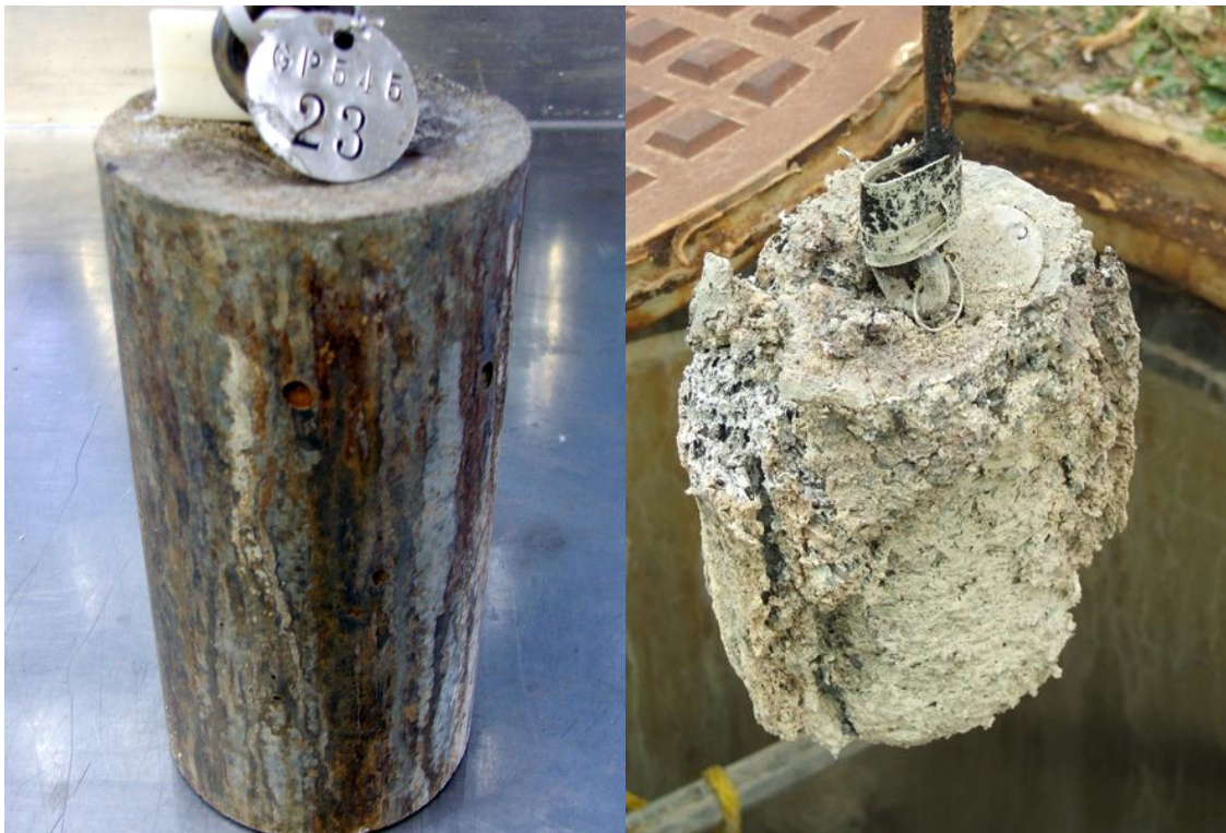
Figure 4.6: Cylinder treated with calcium aluminate premix (left) and untreated cylinder (right) after one year of exposure in a manhole with H_2S > 300 ppm.
