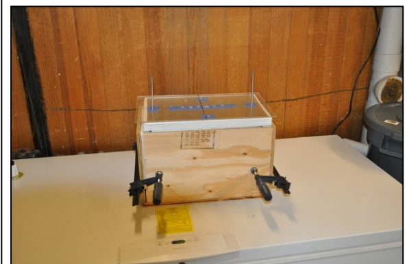
Figure 4-4: Pictures of insulated box container used in both stagnant and low water flow tests
