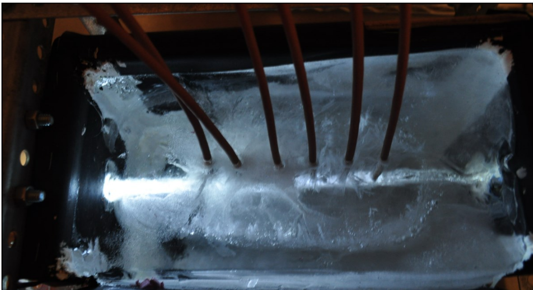
Figure 4-2: Air-filled conduit illuminated through expandable box system after augering conduit to initial dimensions, but prior to the addition of stagnant or flowing water
