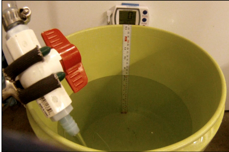
Figure 4-9: GoPro video camera snapshot of outlet reservoir bucket for low water flow experiments. A thermometer and ruler can be seen, as well as water flowing into the outlet reservoir
