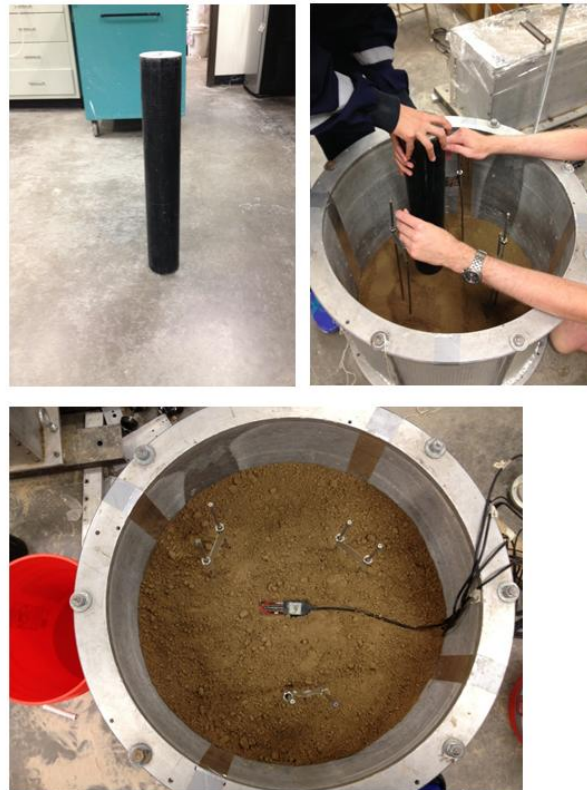
Figure 6.3(a) Compacting rod, (b) Compaction of silt layer, (c) 5TE dielectric sensor placement
