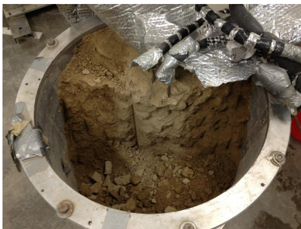
Figure 7.10 Post-test profile section of the unsaturated silt layer showing the drying zone within the heat exchanger array in Test 1
