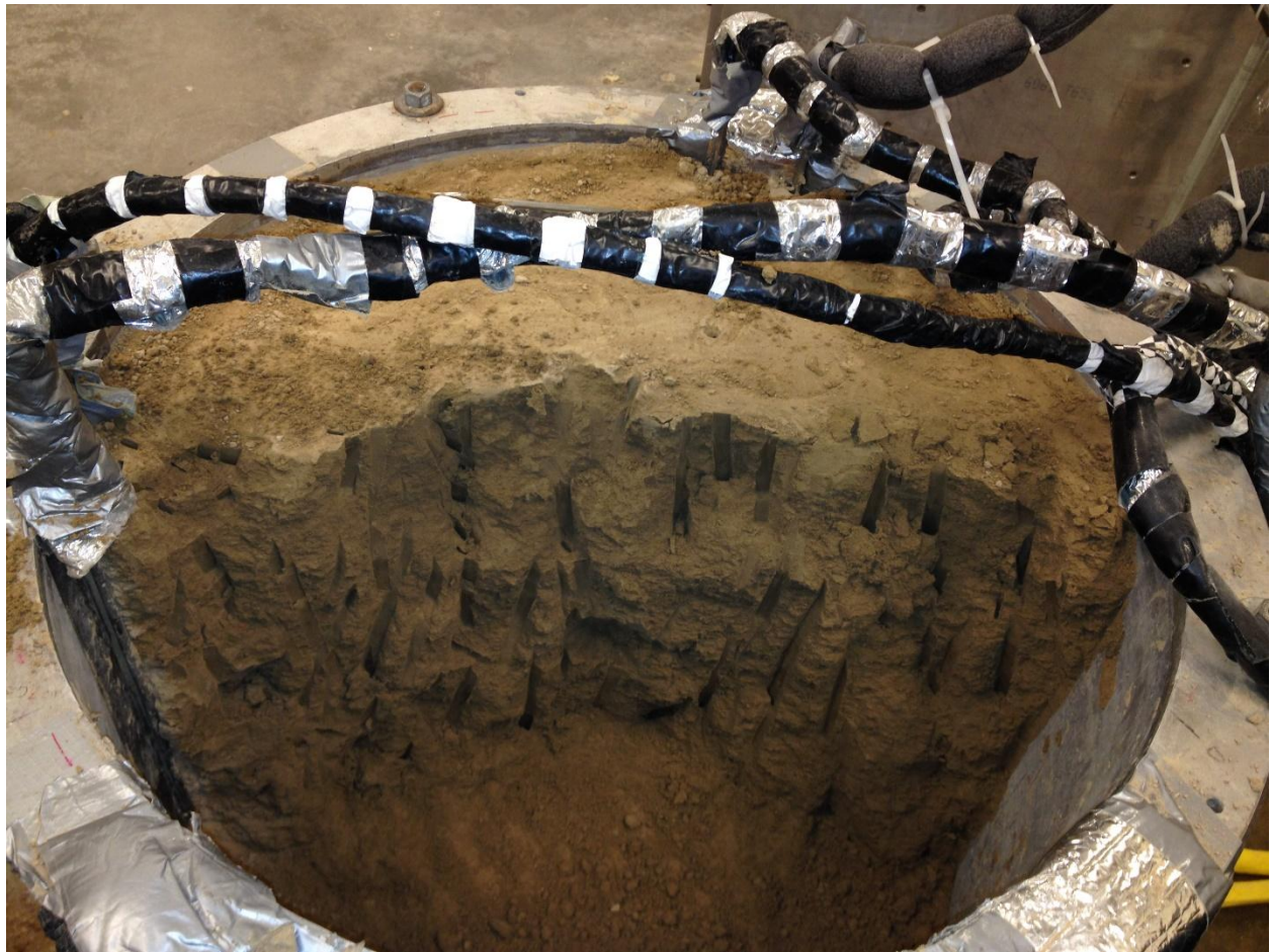
Figure 7.33 Post-test profile section of the unsaturated silt layer in Test 3
