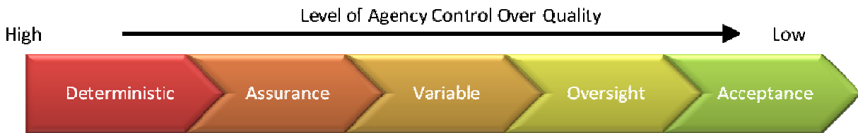
Figure 19 - Spectrum of QAOs and associated levels of project quality control retained by the agency
